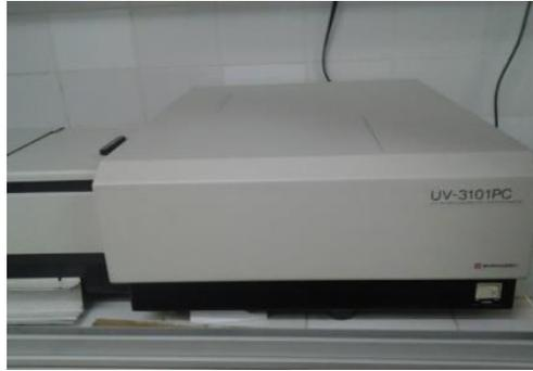
Figure IV.11: Shimadzu 3100 spectrophotometer.
