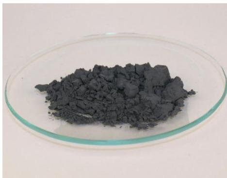
**Figure II.4: Copper Oxide CuO**
