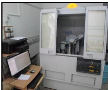
**Figure IV.1: Photograph of the X'pert PRO PANalytical type diffractometer.**
