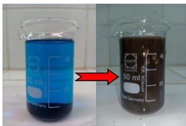
**Figure 1: MB solution with CuO NPs before and after exposition to Ultrasounds.**
