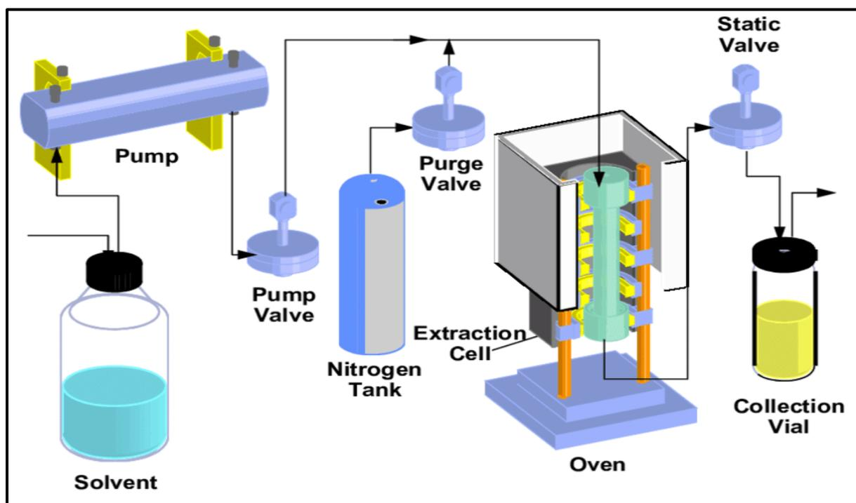
**Figure 11:** Flow diagram of the Accelerated Solvent Extractor 200ä (from: Dionex GmbH, Idstein, Germany) (Van der et al., 1997)
