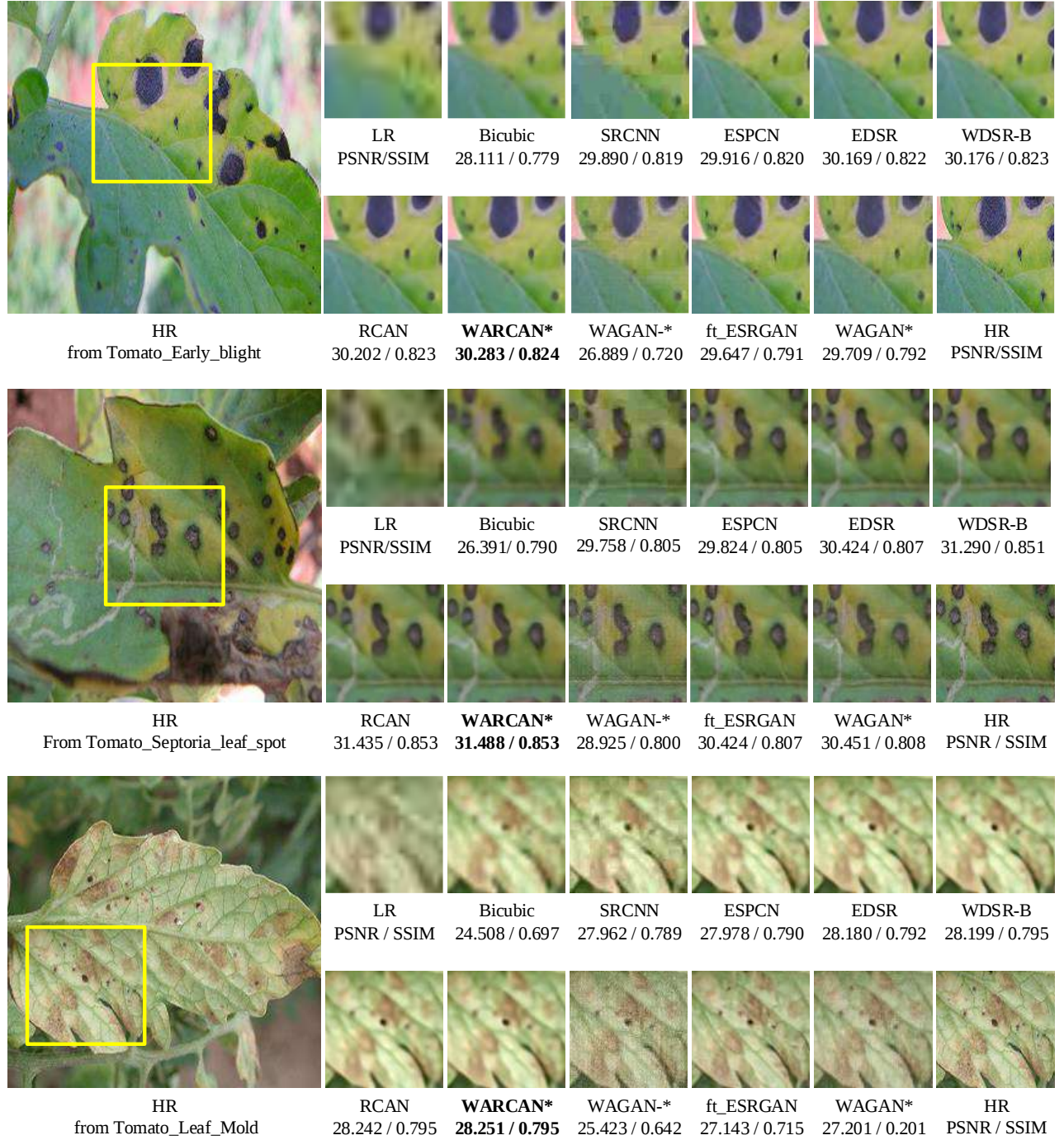
Fig. 4.8 \times 4 reconstruction results of our proposed network compared with LR, state-of-the-art SR images, and reference HR with PlantDoc. (*) refers to our proposed network
