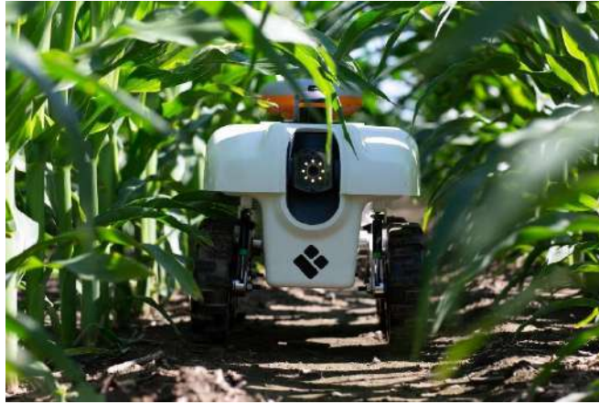
Fig 1.4 Field data collection system "TerraSentia Robot" in the agricultural field [6]
