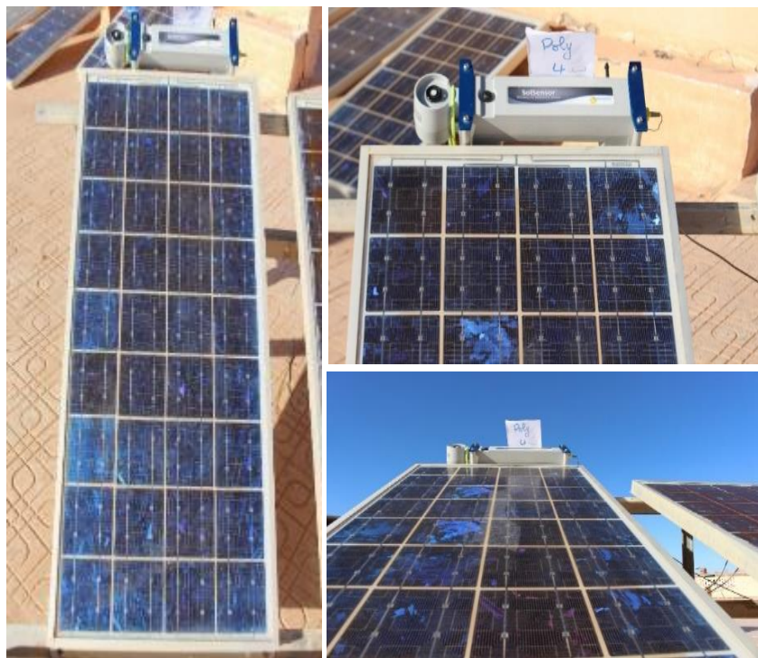
Fig. 3.6 Bus bar yellowing of polycrystalline PV module.
