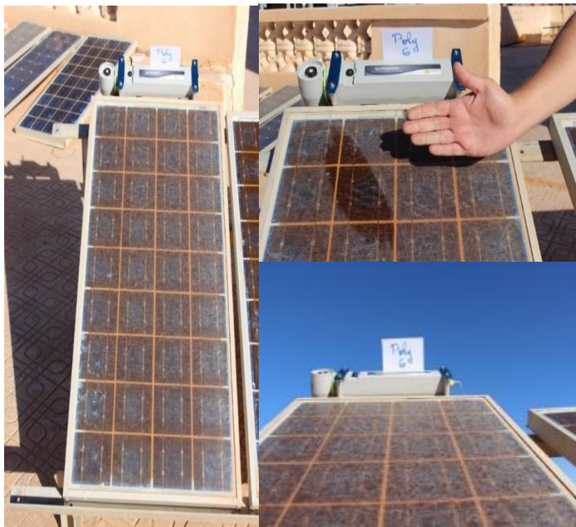
Fig.3.18 Dust deposition on tested polycrystalline PV module
