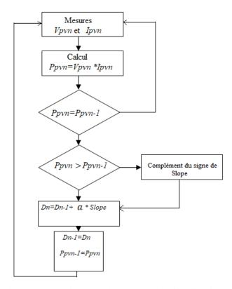
Figure 4.8Algorithme de la commande Hill Climbing.
