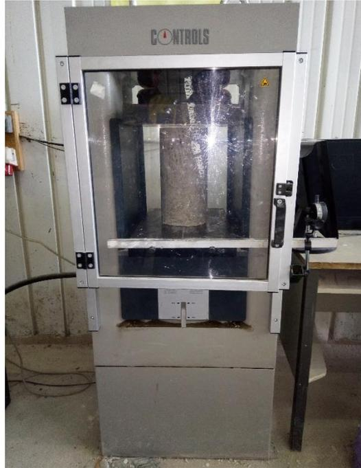
**Photo 4. 1:** Machine (CONTROLS) de compression.
