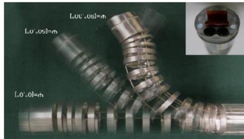
Figure 1.14 : Le robot flexible endoscope.
