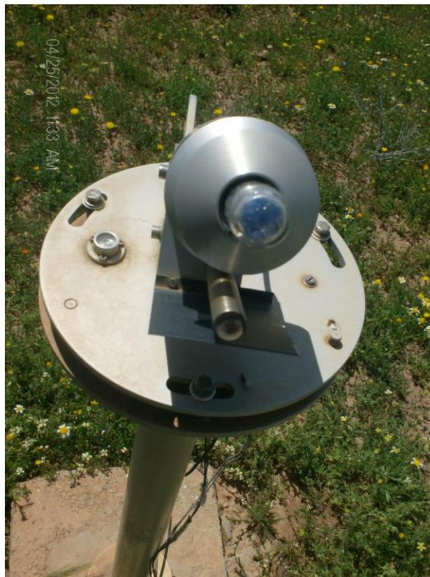
**Figure III.13:** Pyrhelioscope
