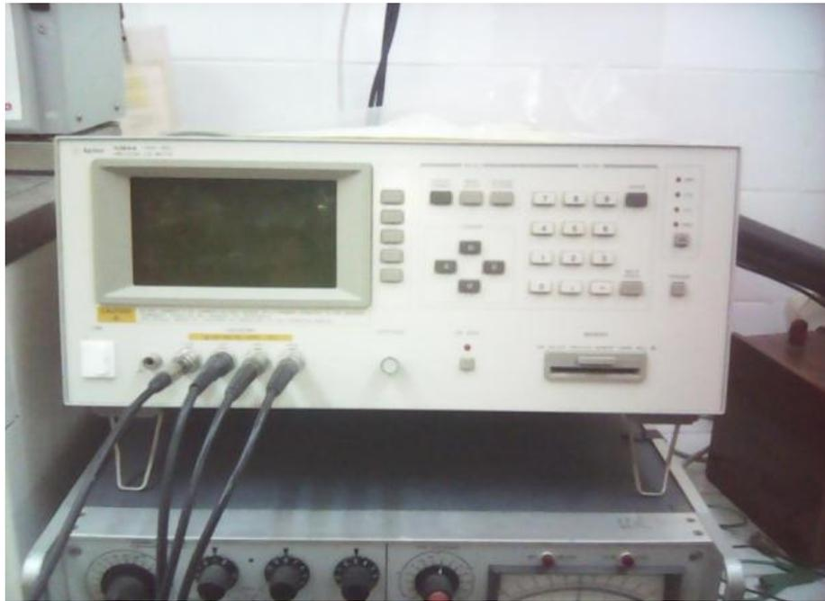
*Figure.II.16. Impedance meter used for C-G-f measurement*
