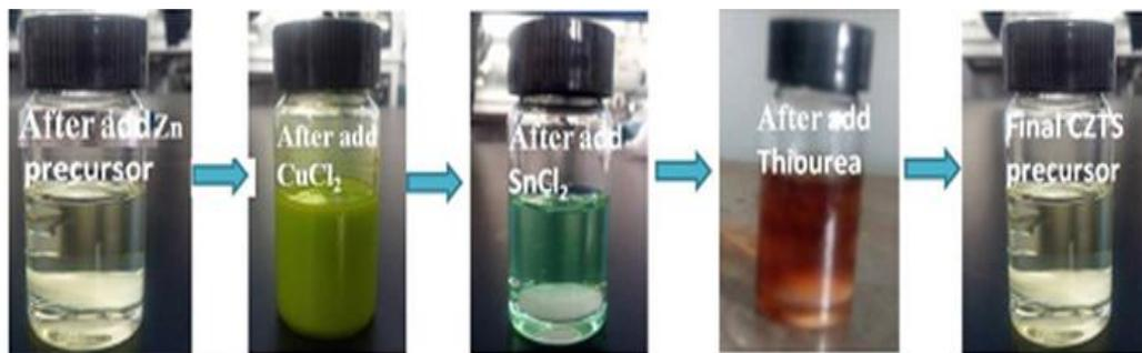
*Figure II.6: The variation of solution color with adding different precursors*
