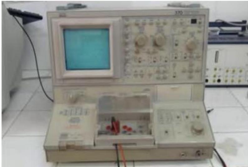
*Figure II.14. Tektronics meter for the I-V measurement*
