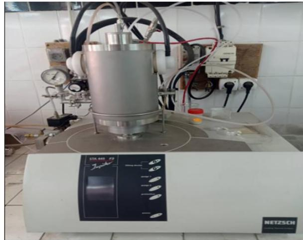
**Figure II.6:** appareil Netzsch (DSC STA 449F3)
