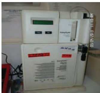
Photo N° 18: EASY LYTE (Na + /k + analyzer).
